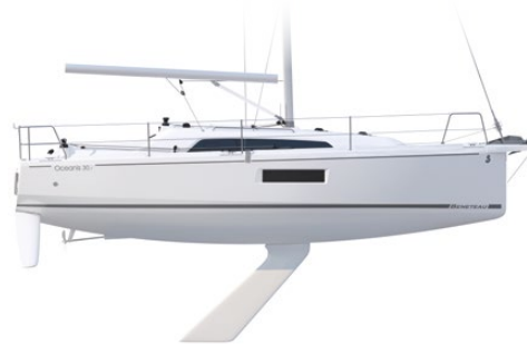
PROFILE Lifting keel version - Quille relevable
